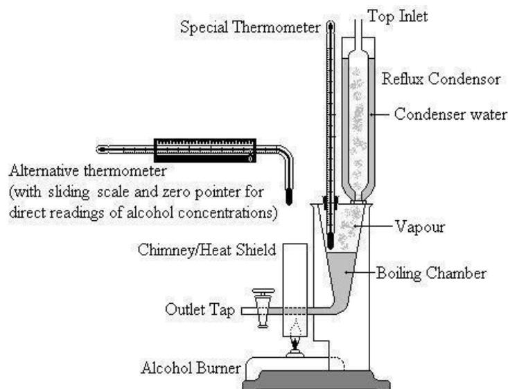
The instrument is usually made of stainless steel and comes in kit form. It may be possible to construct a homemade version of an ebulliometer – the following are crucial requirements:
